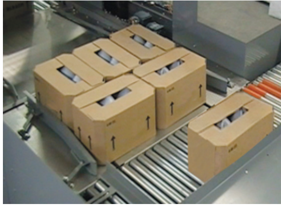
Low level palletizer with extended accumulation table for faster pallet stacking.
